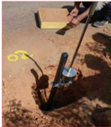
FIELD CBR USING DCPT METHOD IN TRIAL PIT
