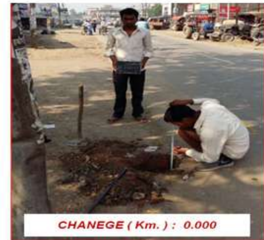
IN-SITU MOISTURE CONTENT AND ROAD CREST MEASUREMENT IN TRIAL PITS
